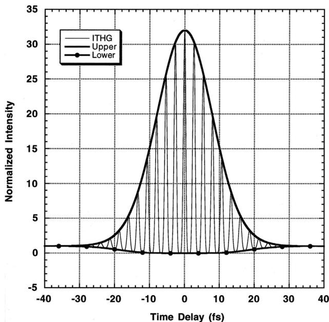
FIG. 3. Calculated third order interferometric autocorrelation for a 20 fs Gaussian pulse.
