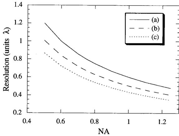
FIG. 6. Lateral resolution of an optical microscope as a function of numerical aperture (NA) based on (a) the lateral position of the first node of the focal field distribution (Rayleigh criterion); or as the FWHM of the lateral focal field distribution in the focal plane from (b) classical theory and (c) full diffraction theory.
