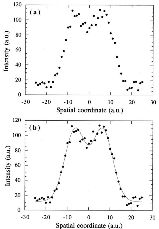
FIG. 7. (a) Intensity profile of two signal point sources, separated according to the Rayleigh criterion, with Poisson noise and 10% detector noise. (b) The use of *a priori* knowledge permits the determination of the position of the two point sources with an accuracy determined by the SNR of the measurement only.
