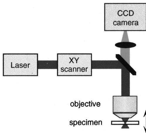
FIG. 5. Generalized schematic of a two-photon absorption microscopy setup. A microscope objective focuses the laser pulses onto the specimen. The specimen is raster scanned in a point excitation mode, generally using mirror scanning for the  $X$  and  $Y$  directions and specimen scanning for the  $Z$  direction. The fluorescence is detected in the backscattering direction and may be imaged directly onto a CCD camera.
