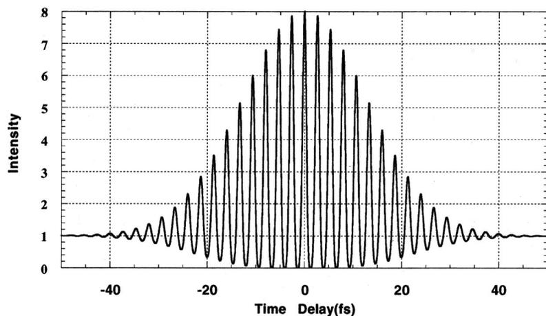
FIG. 2. Calculated second order interferometric autocorrelation for a 20 fs Gaussian pulse.
