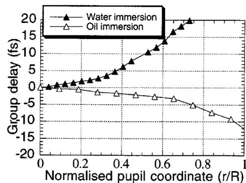
FIG. 4. The radially varying time-of-flight error measured as a function of input radius for an oil immersion and water immersion objective.
