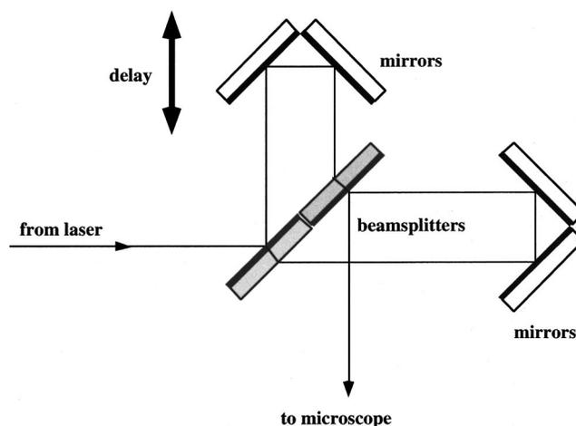
FIG. 1. Basic system for performing autocorrelations.
